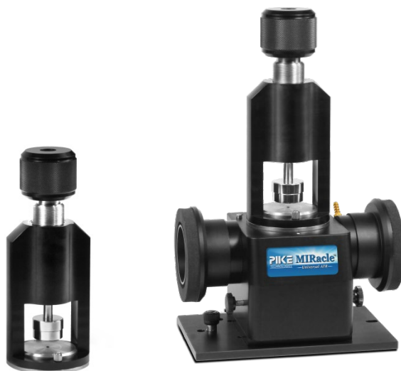
Figure 10. The Sealed High-Pressure Clamp for the MIRacle Single Reflection ATR accessory allows the clamp/crystal plate assembly to be removed from the MIRacle base mounted in the spectrometer to a protective environment for sample loading and handling. Typical applications include studies of toxic or chemically aggressive solids and powders. Dedicated Sealed Sample Chamber Clamp crystal plates, available in diamond, ZnSe or Ge, must be ordered separately.
