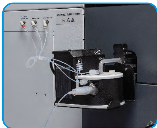
PC 3X installed on Agilent 7900 PC3X-79
