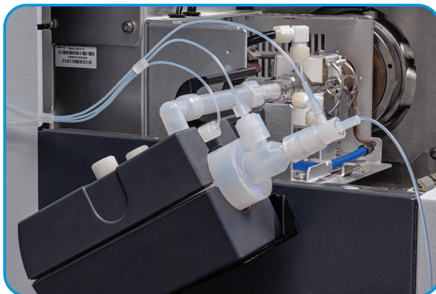
Fluorospray Sample Introduction Kit assembled on Agilent 7900 ICPMS
