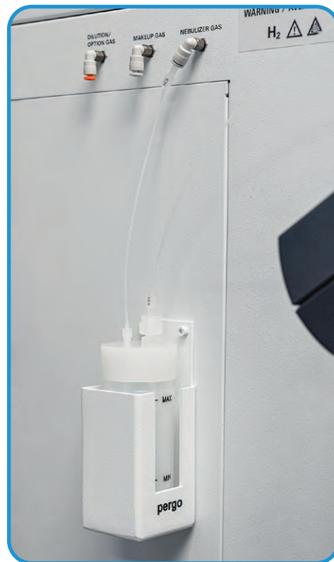
Agilent 7900 with the pergo 500 Argon Gas Humidifier
