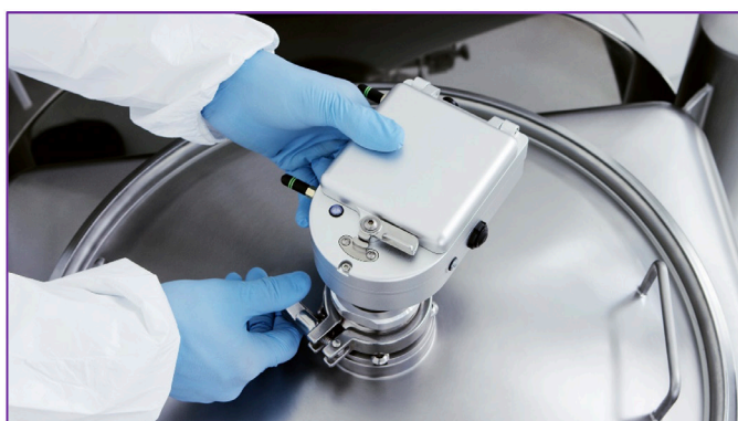
Figure 2. Interface of the MicroNIR PAT-W into the lid of a bin blender
