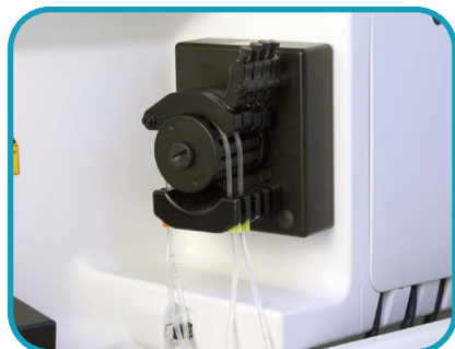
Standard pump on iCAP™ Q/RQ/TQ ICPMS
